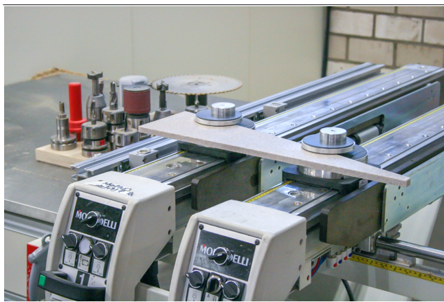
Mechanical clamps VCMC-S4 for clamping wooden parts
